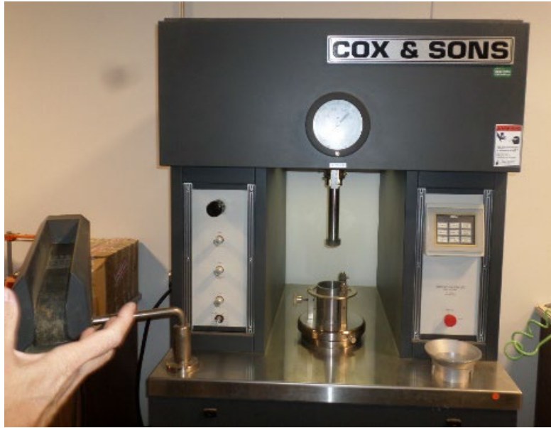
Figure 16. R -value Testing Equipment at CDOT, Pueblo.
